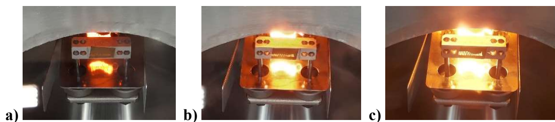
Fig: 6.2: (Mn)-MOF-74 sample under activation at 0.8 A (a), 1.1 A (b) and 1.14 A (c)
